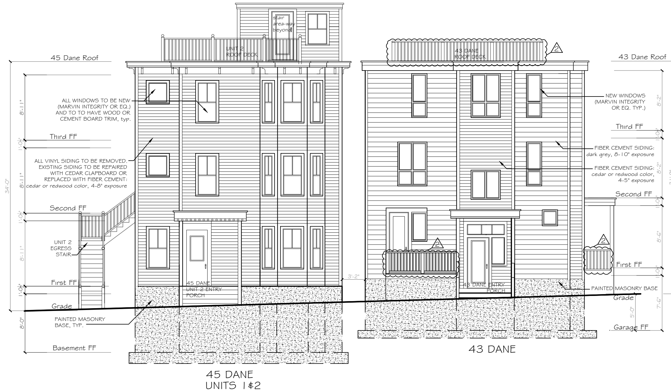
North East / Dane Street Front Elevation
